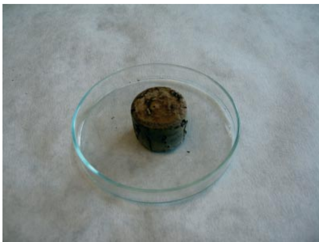
Figure 1. Photographic image of the brown solid obtained after hydrothermal treatment of a mixture of sucrose and ammonia in a Teflon beaker. The porous carbon maintains the shape of the beaker.
